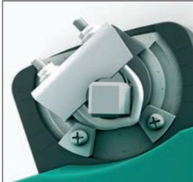
for damper shafts from Ø6 to Ø21mm or from 1/2" to 15/16" (depending on models). The angle of rotation is mechanically limited and it can be adjusted with the turning limiter (depending on models).
